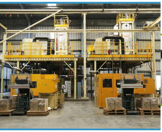
We believe in giving the best product to the client & therefore, manufacture with the world leader solution provide; HUSKY H-PET injection molding machines. We are proud to own 2 Husky H-PET ALL ELECTRIC systems. It deliver us proven, reliable quality by unique technology. To even deliver better, we are soon adding HUSKY HPP 5.0 system too
